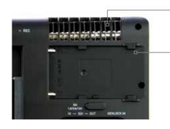
Battery slot Gently slide down into battery slot and lock into position
