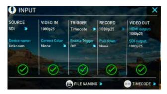
If the camera is Record Run mode, recording can be stopped or started by a moving timecode via HDMI or SDI.
