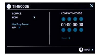
With this setting, the SDI or HDMI input will set the timecode (as long as the source device supports this). The controls to adjust the timecode value are disabled in this setting because the embedded timecode in the SDI/HDMI signal sets the timecode value of the recording. If you want to adjust this please, refer to the manual of your SDI/HDMI input device.
