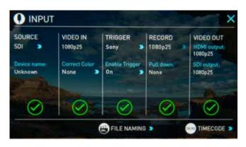
To enable this set TRIGGER to the camera manufacturer in the INPUT
