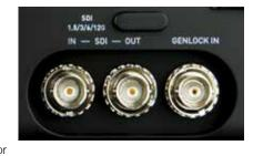
deck is locked to this external reference signal so that the playback output can be synchronized across several playback decks or devices.
